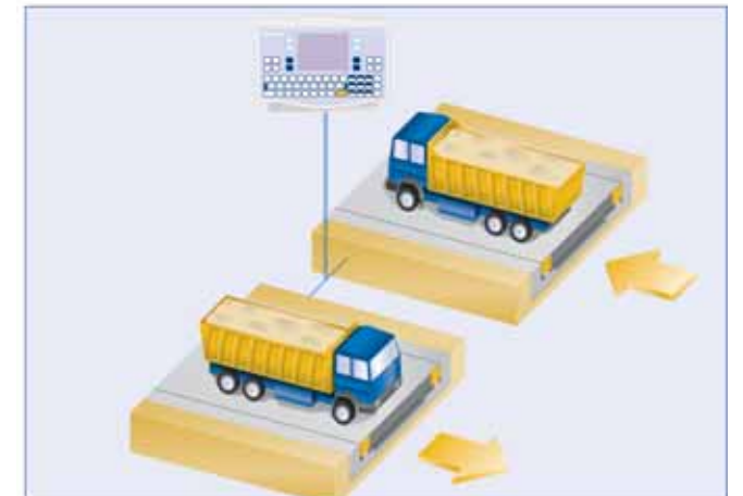
Management of weighing of two platforms with parallel input/output
